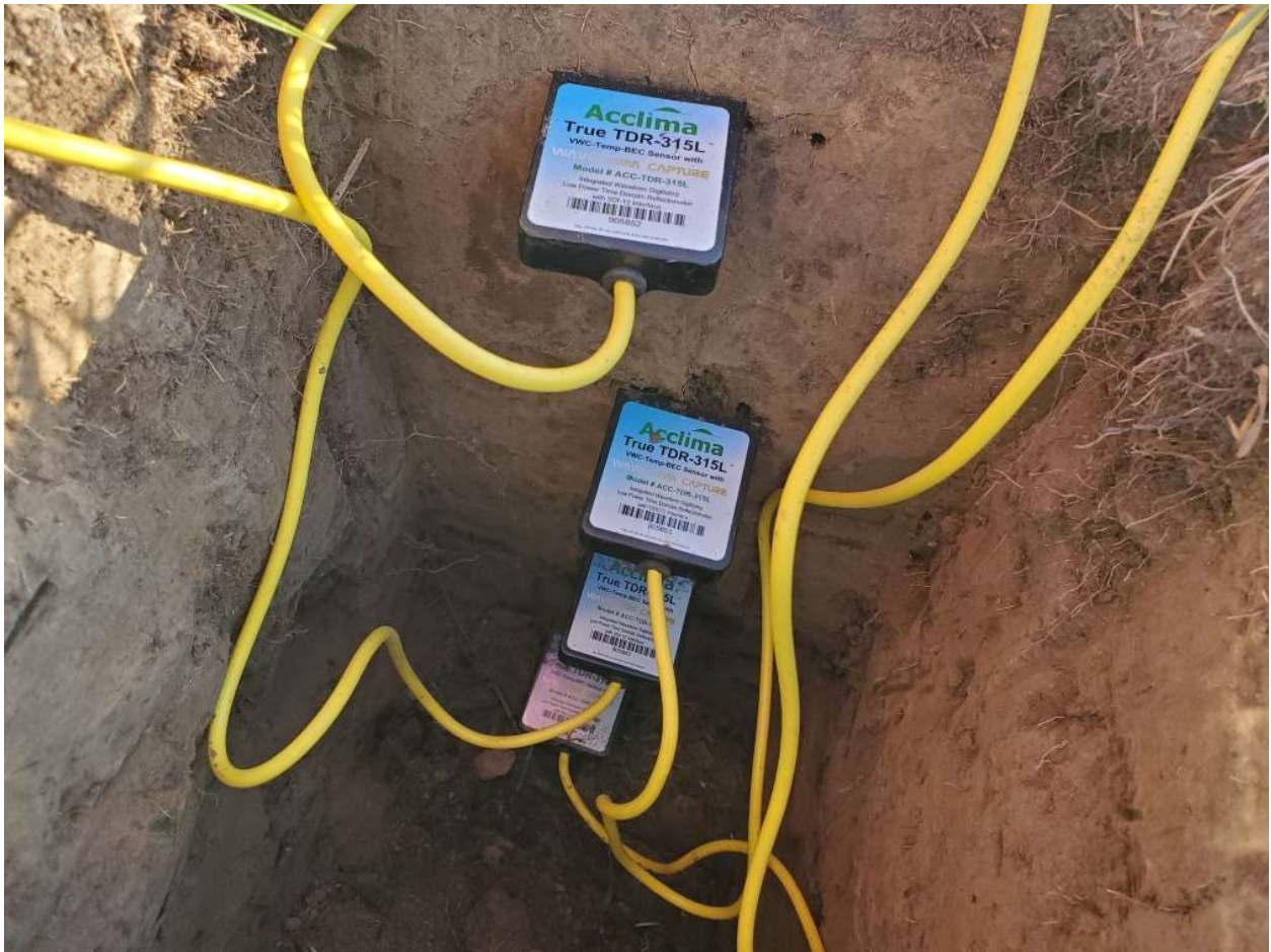
Figure 2.4 Soil moisture sensor installation representing depths of 0-12, 12-24, 24-36, and 36-48 cm below the soil surface.
