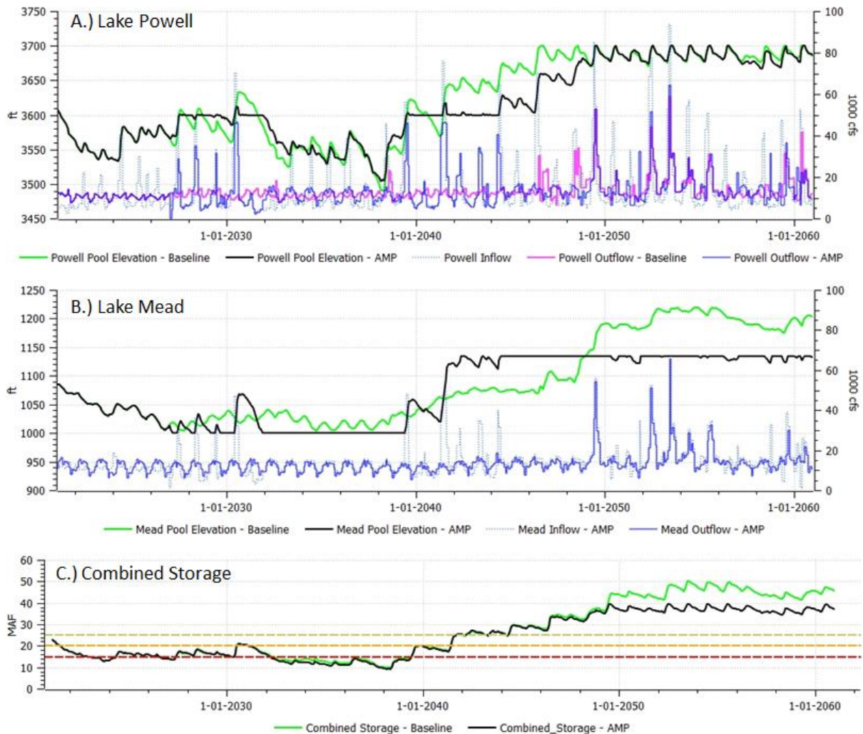
Figure 9.9. Reservoir characteristics comparing baseline and the FMF-B2 AMP with a sample Dry to Wet hydrology. (A) shows Lake Powell elevations, inflows, and outflows. (B) shows Lake Mead elevations, inflows, and outflows. (C) shows combined storages with shortage thresholds.
