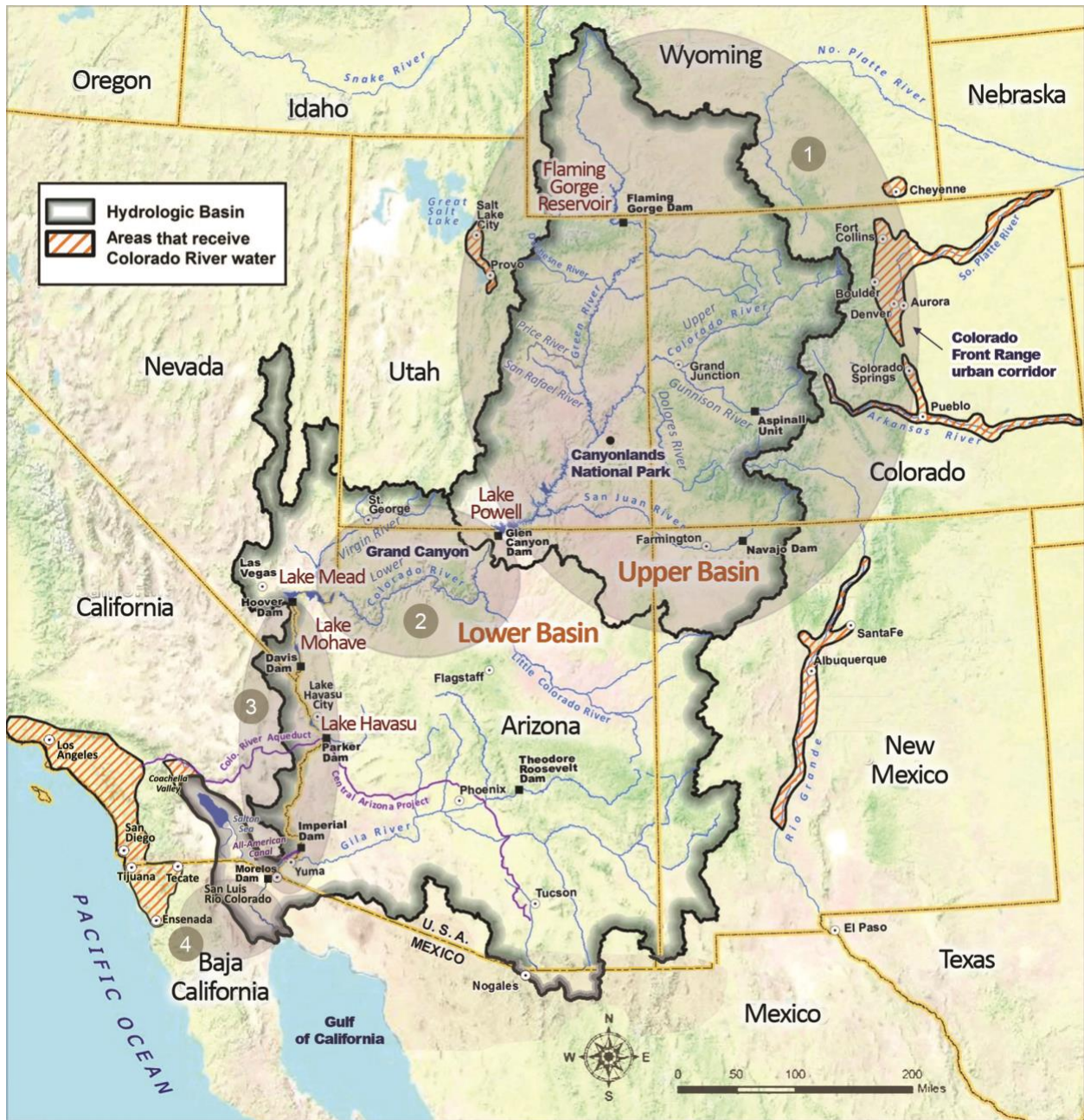
Figure 2.1. Map showing the Colorado River Basin and surrounding areas that use Colorado River Water. Four regions are delineated, based on the degree to which flow is regulated and the channel physically manipulated: 1) the Upper Basin, 2) the Grand Canyon, 3) the lower river between Lake Mead and Morelos Dam, and 4) the Delta. The base map was adapted from Reclamation’s 2012 Basin Study (USBR, 2012) to include the entire Colorado River delta and Salton Trough within the United States and Mexico. This map also shows the areas in Mexico outside the watershed that are served by Colorado River water.
