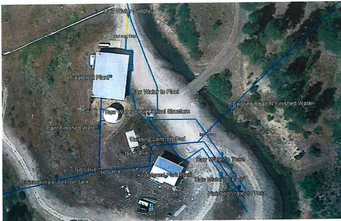
Figure 5. Close-up of Figure 4; Plant-scale detail of existing major infrastructure, including abandoned lines (yellow).
